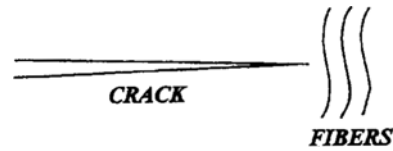
Fig. 3 Fibers located ahead of the crack tip.
